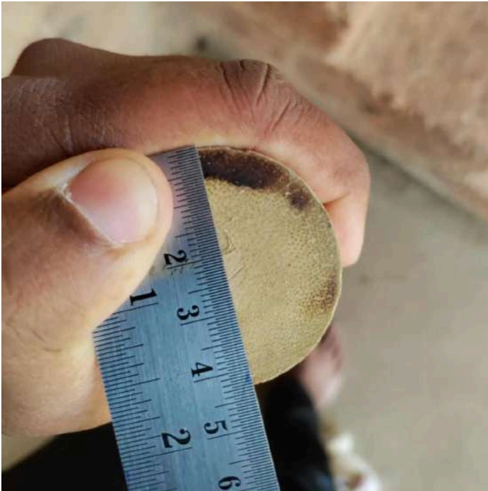
Diameter of Manga Bamboo 43 \text{ mm} = 4.3 \text{ cm} = 1.70 \text{ inch}
